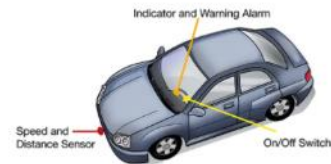
Parts of a typical forward collision warning system
